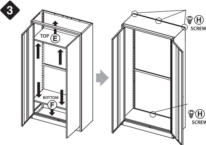
**Pic 3:** Install (E) TOP & (F) BOTTOM into body of cabinet and fix using (H) SCREWS
