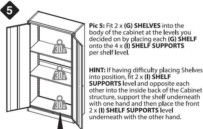
**Pic 5:** Fit 2 x (G) SHELVES into the body of the cabinet at the levels you decided on by placing each (G) SHELF onto the 4 x (I) SHELF SUPPORTS per shelf level.
