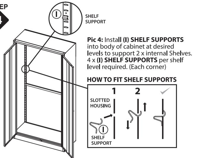
**Pic 4:** Install (I) SHELF SUPPORTS into body of cabinet at desired levels to support 2 x internal Shelves. 4 x (I) SHELF SUPPORTS per shelf level required. (Each corner)
