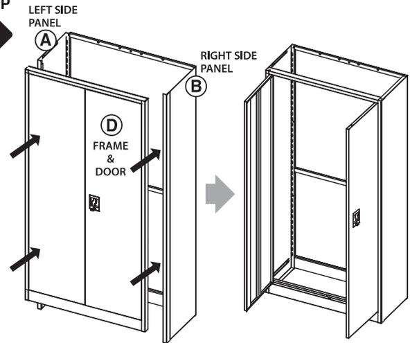
**Pic 2:** Join (A) LEFT SIDE PANEL & (B) RIGHT SIDE PANEL with Frame by clipping FRAME & DOOR (D) into (A) & (B) from inside standing structure.
